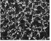
Membrane filters allow the efficient retention of submicron particulates and organisms.
