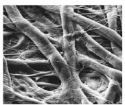
Whatman cellulose filter papers exhibit particle retention levels down to 2.5 µm.
